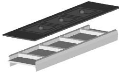
Figure 1. "Ladder box" test part and PCB with three antennae for cavity to cavity shielding.
