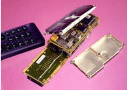
Figure 4. Small plated plastic shielding covers mount directly onto PCB ground traces. Covers provide EMI isolation between circuits and prevent the escape of radiated emissions.
